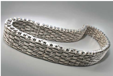
LuK pull-chain (above) and Jatco push-belt (above right): two CVT alternatives
